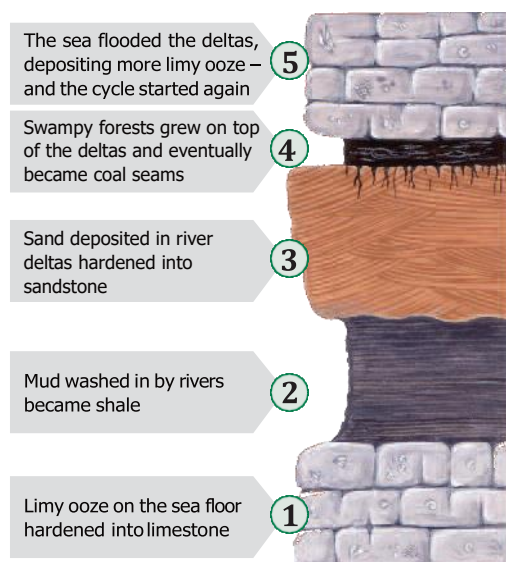
A highly simplified section through a typical Yoredale cyclothem with interpretations of the conditions under which each rock type formed: © Elizabeth Pickett
